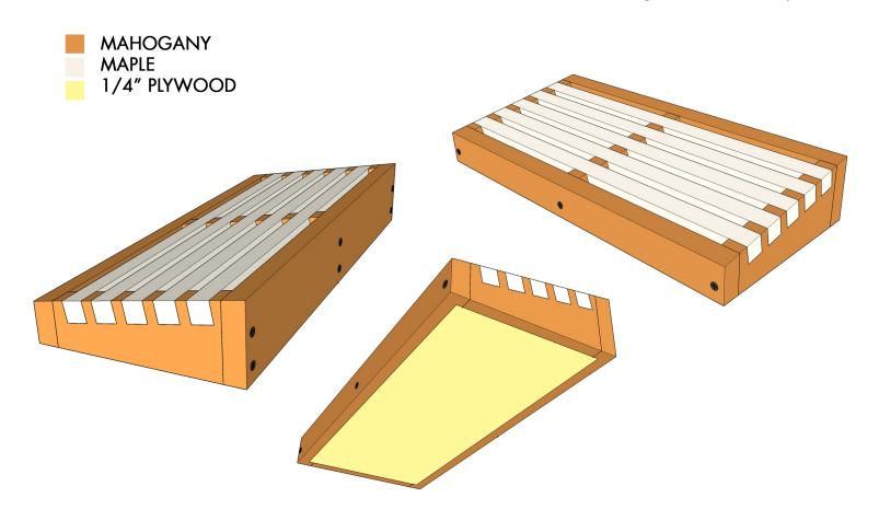
**Not Shown:** Drill a hole in the bottom plywood for routing power adapter cable. Add 4 rubber feet and a handle to the back. Use small screws to attach plywood. Round over the edges, counter-sink the screws and add wood plugs for a cleaner look.
